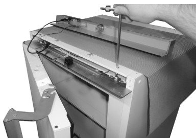
39. Tighten the two M8 screws in the top bracket
