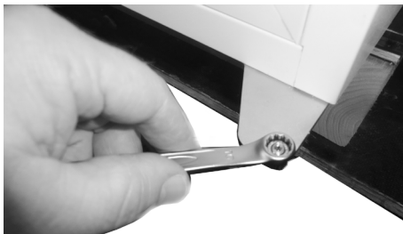
24. Remount and tighten pivot nut
