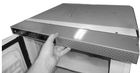
40. Carefully push the top panel back into position
