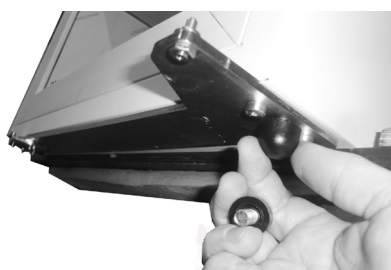
18. Remove the two front feet
