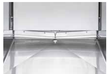
Test room bottom with slope to the condensate drain.
