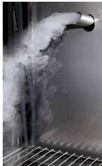
Aerosol mist without heat introduction into the test room.
