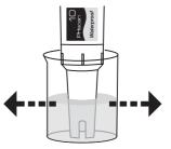
8. Dip electrode about 2 to 3cm into the pH4.01 (or pH10.00) buffer solutions and stir slowly.
