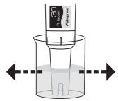
8. Dip electrode about 2 to 3cm into the pH4.00 (or pH10.00) buffer solutions and stir slowly.
