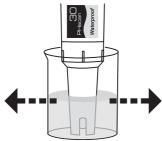
3. Dip the probe into the solution, stir slowly. Wait 3 to 5 seconds to let the reading stabilize. The measurement is finished.
