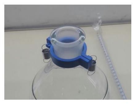
Assemble clamp on bottle neck, & place springs on possition
