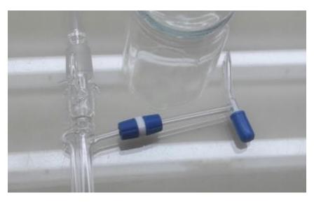
Joint both tubes with center part of adapter. Tighten screw to avoid leakage.
