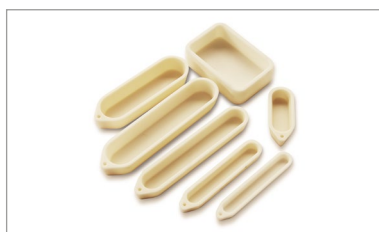
For loading samples, sample boats and crucibles are available in various sizes and materials.
