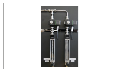
With automated gas valves
