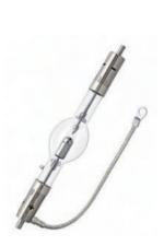
The metal halide lamp is imported from Germany OSRAM. The spectral curve of this series of metal halide lamps is very close to the solar spectrum, which can simulate the radiation environment of sunlight.
