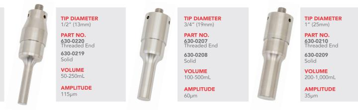
When driven at its resonant frequency, the probe expands and contracts longitudinally about its center. The distance the probe moves is measured as the amplitude. The greater the mass ratio between the upper section and the lower section, the greater the amplification factor, and the greater the peak-to-peak excursion at the tip of the probe. The amplitude setting can be adjusted on the power supply.
