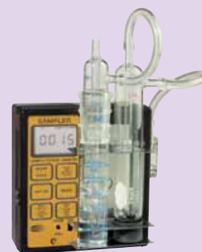
Glass Trap shown with Impinger and PCXR8 Sample Pump
