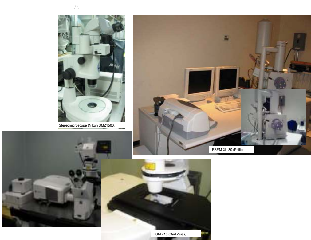
Figure 2 Different kinds of microscopes applied in the study of food microstructure. A) Stereomicroscope, B) Environmental Scanning Electron Microscope, C) Confocal Laser Scanning Microscope.
