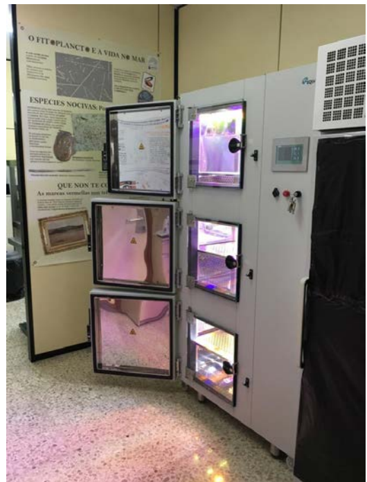
Lighting device employed for the setting of different light intensities and spectral qualities, with 6 independent LED channels control.
